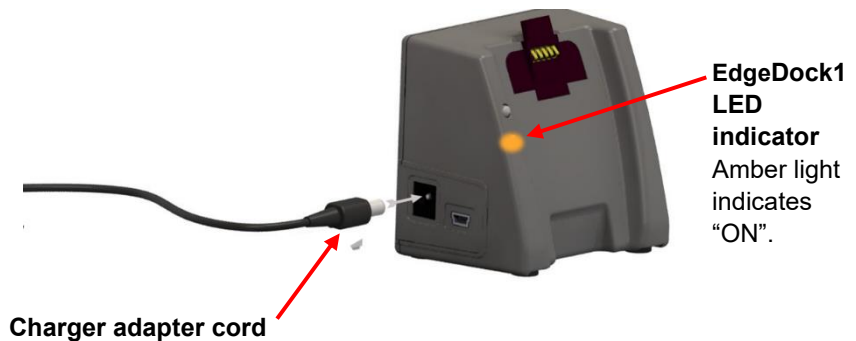
Figure 2-7 Attaching charger adapter to EdgeDock1 and EdgeDock5
