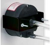
Mounting hardware is supplied with the Minihelic<sup>®</sup> II gage for panel mounting through a single hole, 2-5/8" (67 mm) in diameter. Panel thickness up to 1/2" (13 mm) can be accommodated with the hardware supplied. If necessary, surface mounting of the gage can be accomplished by means of two 4-40 screws into the tapped mounting bracket stud holes in the rear of the gage. Surface mounting requires clearance holes in the panel for the two pressure taps.
