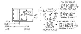
SERIES 2-5000 Minihelic® II Differential Pressure Gages have clean design, small size, low cost and sufficient accuracy for all but the most demanding applications. With housing molded from mineral- and glass-filled nylon and a lens molded from polycarbonate, this gage will withstand rough use and exposure, as well as high total pressure up to 30 psig (2.067 bar). Over-pressure is accommodated by a blow-out membrane molded in conjunction with the diaphragm.
