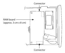
(9) Remove the battery connector from the RAM board.
