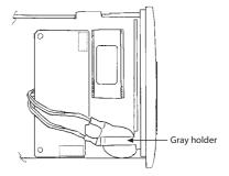
(13) Insert the body into the case. Do not exert excessive force if the body cannot easily fit into the case. Also, make sure that the boards mounted on the body are not loose or twisted.
