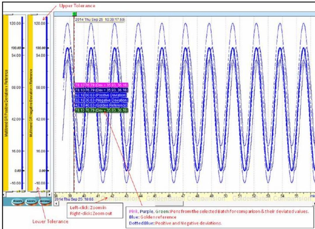
Figure 4: Golden reference value and Golden batch comparison
