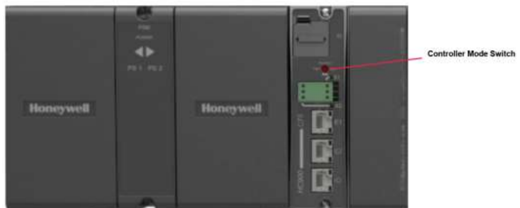
Figure 4 Redundant Controller on 900R01
