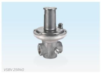
Relief valve for relieving brief pressure surges in control systems thus preventing the safety shut-off valve JSAV from being activated unintentionally. The VSBV reduces too high a pressure increase due to gas creeps which are the result of gas pressure regulators that are not tight closing.
