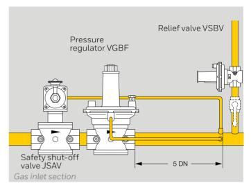
Relief valve VSBV relieves pressure peaks thus preventing the safety shut-off valve JSAV from being activated unintentionally.
