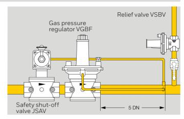
If the controls downstream of a gas pressure regulator are not resistant to the supply pressure, EN 746-2 prescribes a safety shut-off valve upstream and a relief valve downstream of the gas pressure regulator – regardless of how high the inlet pressure is.
