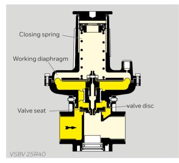
Relief valve VSBV is closed by a spring when no pressure is applied.
