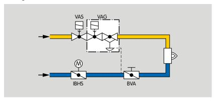
The safety closing function ensures that in the event of a mains voltage failure air cannot stream into the furnace without being under control.
