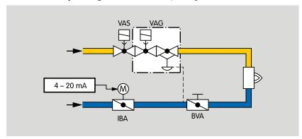
In pneumatic ratio control systems, the butterfly valve with mounted actuator IBA determines the air volume for the required burner capacity.
