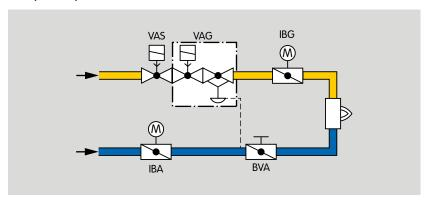
If the burner is to be operated with excess gas or air for reasons of process operation, the butterfly valve with actuator IBG can be used to correct the lambda value.
