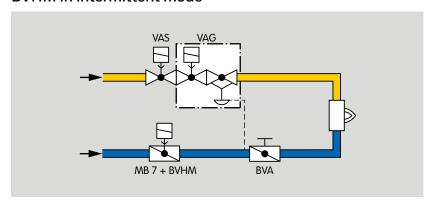
Solenoid actuator MB 7 and butterfly valve BVHM are used for intermittent switching of the burner.
