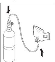
1. Connect a tube from a cylinder of calibration gas to the calibration cap's right spigot.
