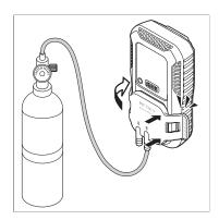
2. To attach the calibration cap to the gas detector, hook the cap's left clip to the corresponding groove of the detector and snap the right clip into place.
