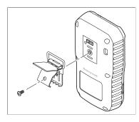
If the belt clip is damaged or loose, replace it with a new one. Insert a screwdriver through the hole in the clamp and loosen the screw to detach the clip. Put a new clip in place and fasten it.
