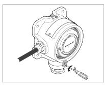
4. Loosen the grub screw on top of the sensor cover.
