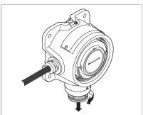
5. Turn the sensor cover counterclockwise to remove it.
