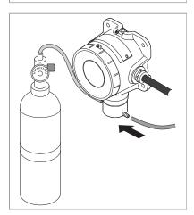
3. Connect another tube to the other gassing port, and place the end of this tube in a position so that gas can exhaust safely away from the work area and other personnel.
