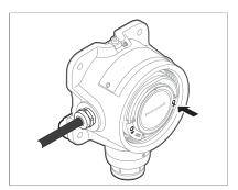
Press and hold the UP button for 10 seconds to switch to sensor replacement mode. In this mode, the detector output is inhibited and the sensor circuits are internally isolated.
