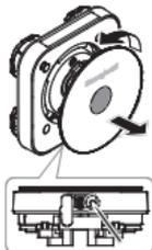
1. Remove the front cover from the detector module to expose the retaining screws as follows:
