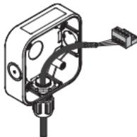
4. Connect the cable to the appropriate terminal block, referring to section 2 to 4 depending on the version. Strip and insert the end of each wire into the corresponding terminal hole, and tighten the terminal screw, using a flat-blade terminal screwdriver until the wire is secured.
