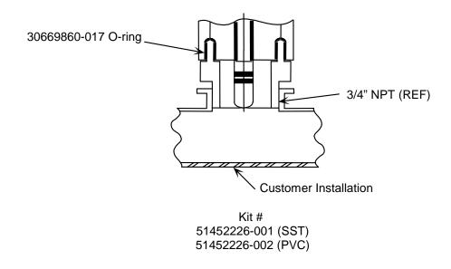
Figure 3-5 In-Line Mounting Kit
