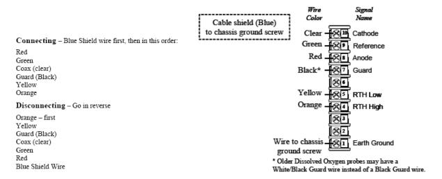
Figure 3-3 Connect/Disconnect Sequence for the DO Probe with an Integral Cable and the UDA2182
