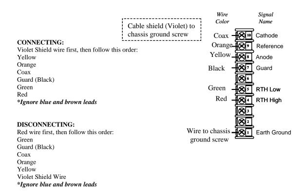
Figure 3-4 Connect/Disconnect Sequence for the DO Probe with Quick Disconnect Option and the UDA2182
