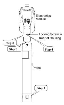
Figure 3-1 Integral Mounting
