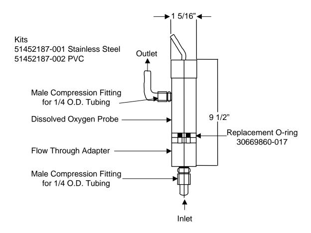
**Figure 3-6 Flow Through Mounting**
