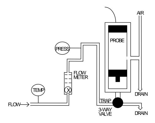
Figure 3-7 Mounting Recommendation for Easy Calibration in Boiler Control Loop
