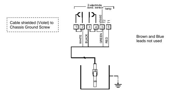
04973 series cells with integral cable leads connected to an APT4000
