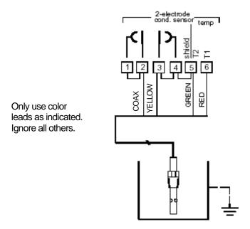
Figure 4-6 Wiring Diagram for 4973 Cells with Quick Disconnect Cable Connected to APT4000
