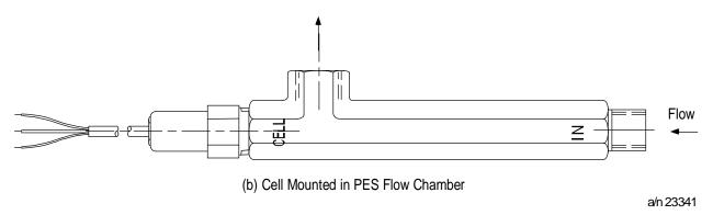
Figure 1-3 Two Piping Arrangements for the Cell
