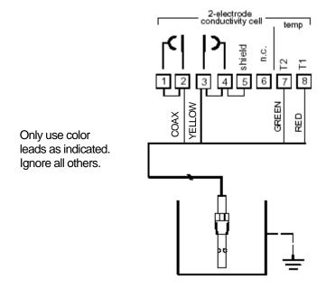
Figure 4-7 Wiring Diagram for 4973 Cells with Quick Disconnect Cable Connected to APT2000
