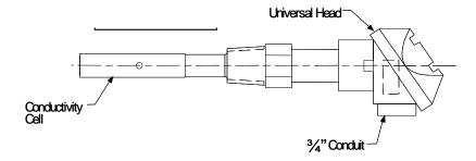
Figure 1-1 4973 Type Conductivity Cells, for Flow and Insertion-type Applications.
