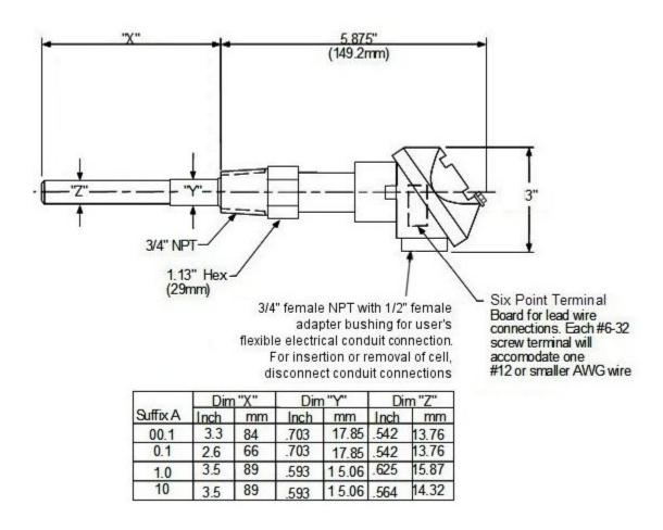
Figure 3-3 Outline and Dimensions for Conductivity Cell with Universal Head
