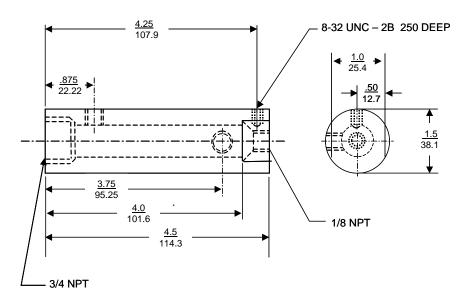
Figure 3-2 Dimension Drawing for 31079198 Flow Chamber
