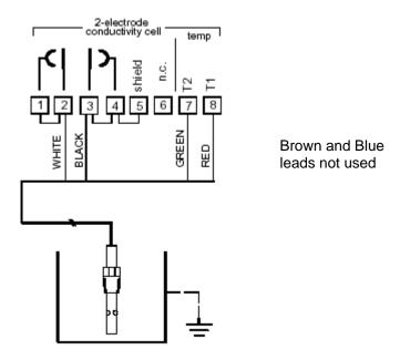
04973 series cells with integral cable leads connected to an APT2000
