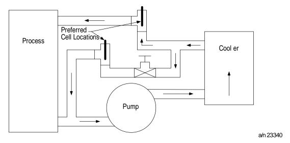
Figure 1-2 Recommended Locations for Mounting a Conductivity Cell
