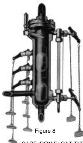
Figure 8 CAST IRON FLOAT TYPE COLUMN REVEALING INTERNAL FLOATS. COLUMN IS EQUIPPED WITH A DIRECT READING TUBULAR GLASS WATER LEVEL GAGE.
