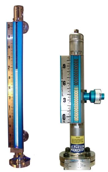
The Jerguson Magnicator is designed to safely determine the level of liquids and liquid interfaces. The operation of the Magnicator is both simple and unique. The patented magnetic circuit provides the best combination for floats and indicators available. The magnets in the float actuate the indicator flags as the level rises or falls. The indicator tracks the float exactly, which in turn provides an accurate level measurement.
