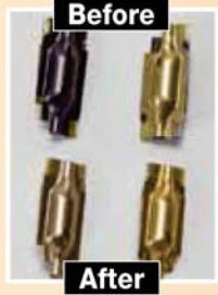
Heat has faded these anodized aluminum flags to make them nearly indistinguishable.
