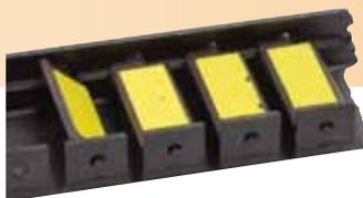
Weak magnetic coupling between the flags and float magnetic field can lead to missed flags and unreliable indication. Operator must manually “reset” the flags or wait for the level to cycle.
