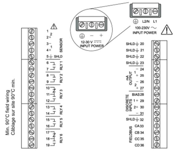
In case of power failure, all relays will fail in their de-energized states.
