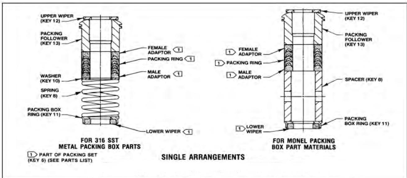
Figure 2: PTFE V-Ring Packing Arrangements for Plain and Extension Bonnets
