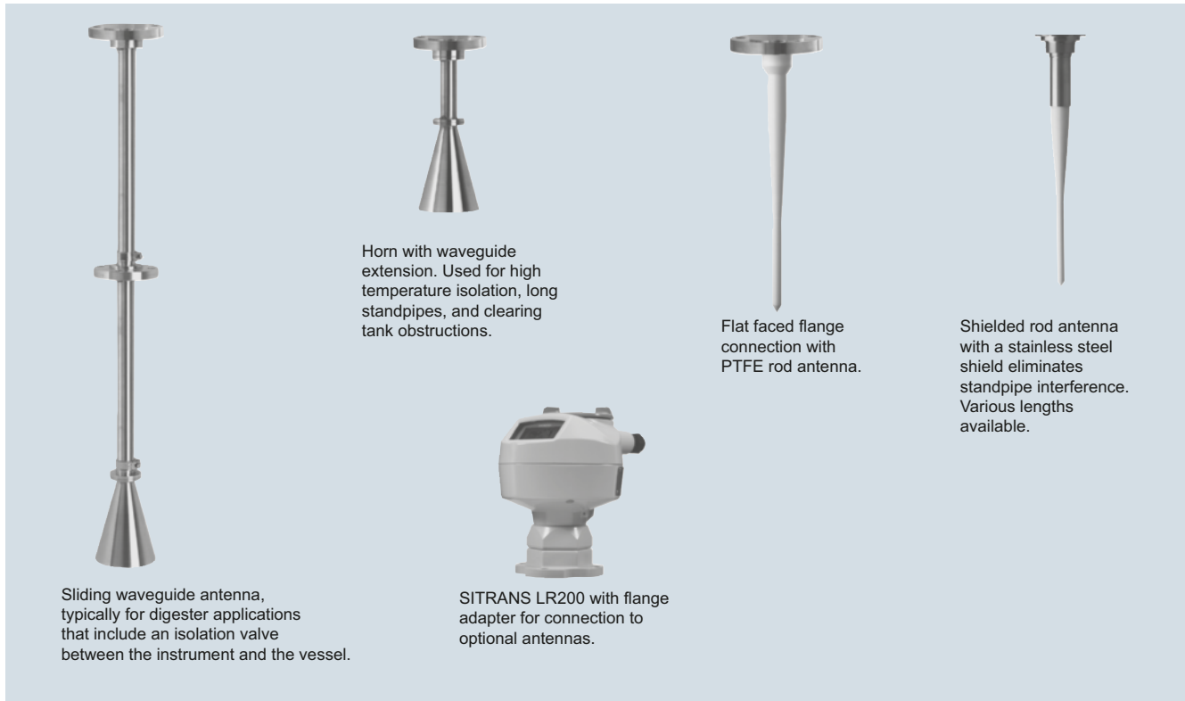
Antenna configurations for SITRANS LR200
