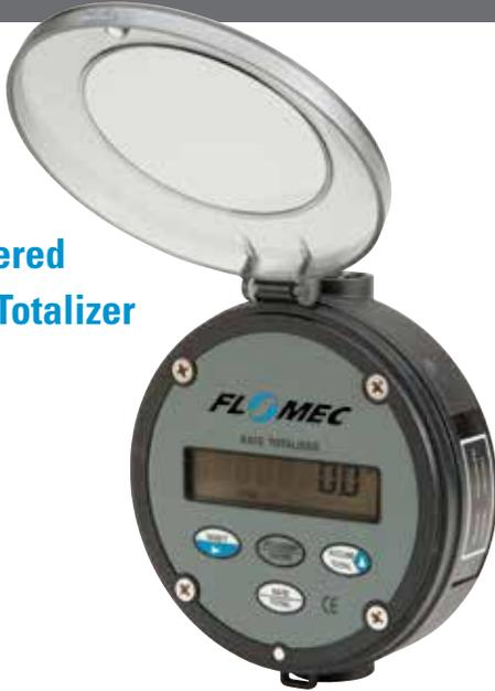
FLOMEC® LCD display RT12 is a fully programmable self-powered flowrate totalizer specifically designed for computing and displaying flowrates and totals from flowmeters with pulse, sine wave or frequency outputs.
