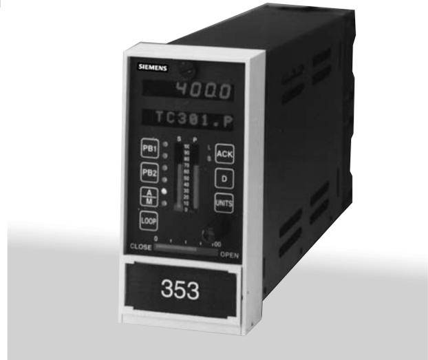
as an integral element in a plant system. Loops are configured for control, sequence, or logic as needed within the Model 353. Each configured loop can have a virtual operator display that is viewed locally using the LOOP button on the faceplate and is mapped to network communication for a plant operator station. Alarm management is handled using the L (Loop) & S (Station) indicator lights along with the priority assignments and flashing options of each alarm.
