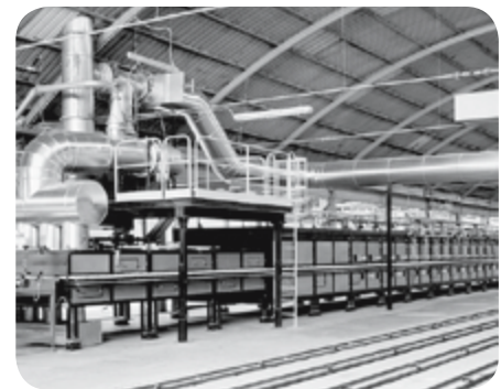
Roller hearth kiln in the ceramics industry
