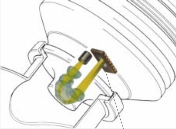
A light source transmits light against the interface between a prism and the process solution. The light rays meet the surface at different angles.
