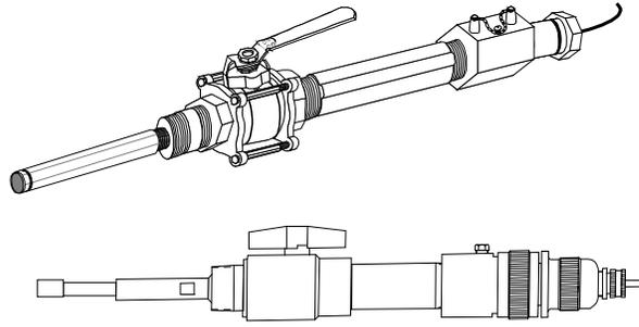
**Top: 4909 SS Insertion/Removal Cell Assembly**
