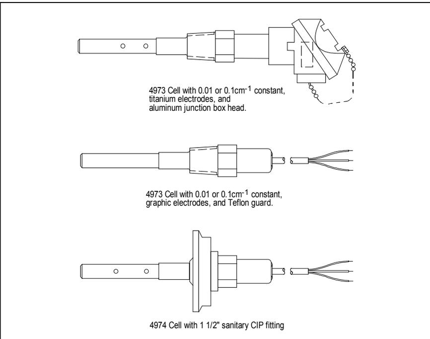
The cells have been designed to keep the electrodes and the temperature compensator immersed in the stream flow, ensuring that the cell will respond quickly and accurately to changes in both solution concentration and temperature.
