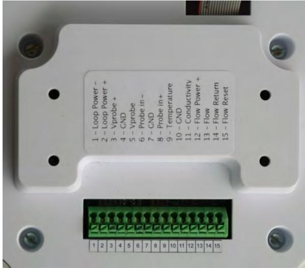
Figure 3-2 - This view of the inside of the front cover shows the connector for the probes. The label in the middle lists the connections.
