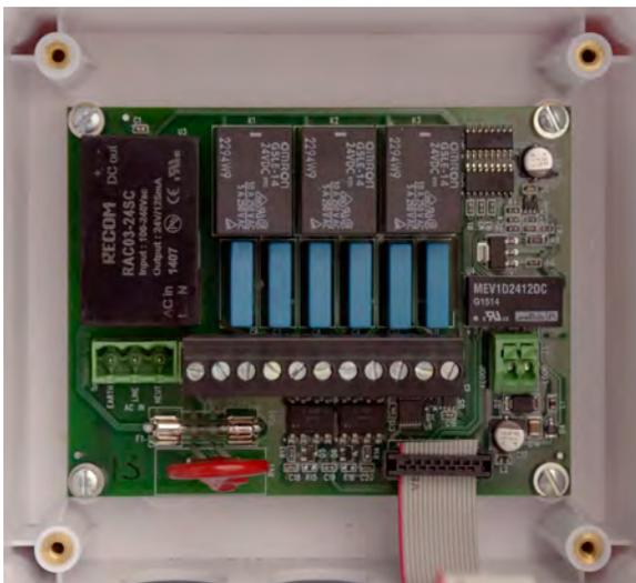
Figure 3-3 - Power circuit board showing relay connector and relays. The second 4-20 mA output is also on the board.
