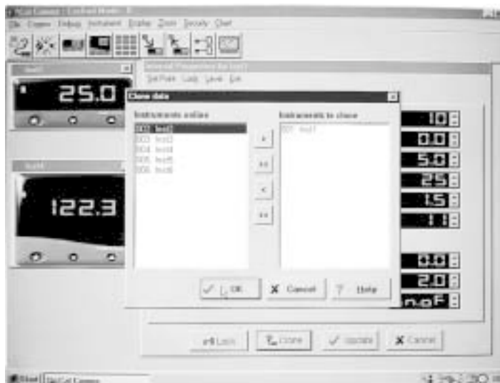
Copying settings from one instrument to another or others significantly speeds up instrument configuration for multi-zone applications.
