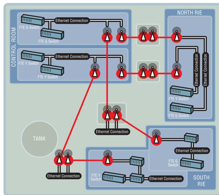
Extending the control network to remote enclosures provides an efficient and reliable way to automate more areas of the plant.
